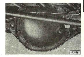
Unscrew rear axle housing cover and remove it together with gasket.
