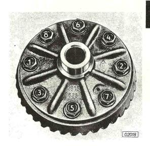
Check lateral runout of installed ring gear in V-blocks. Max. permissible runout = .0031 in. (0.08 mm).
