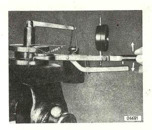
Measure width of both differential side bearings, using gauge S-1065 and measuring scissors. Prior to taking measurement rotate bearing a few times, then suspend a 2.2 lbs. (1 kg) weight from gauge lever so that bearings are properly preloaded.
