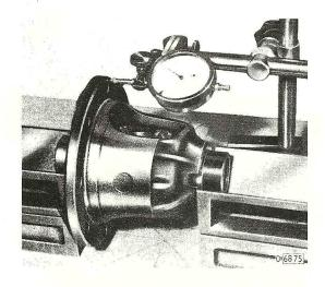
Place differential case in V-blocks and check axial runout of ring gear contacting area.
