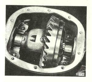
The markings are required to determine the smallest width between differential case and rear axle housing.
