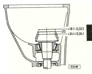
The hex nut in front of the slotted sleeve is self-locking and need not be secured. Therefore always use a new nut.
