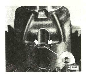
Drive lock pin into pinion shaft and secure.
