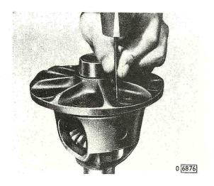
With a suitable drift drive lock pin from ring gear side out of pinion shaft.
