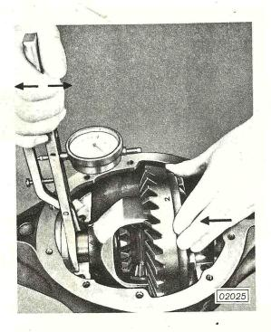
Then measure width on opposite side of differential while pushing differential case with ring gear against drive pinion. There must be no backlash. The width on differential case side has to be measured at the marking at which the smallest width on ring gear side was established. Write down value obtained.
