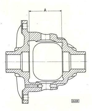
Due to the different measure "A" of 2326 in. (59.08 mm) on differentials with the catalog no. 4 10 213 and 4 10 222 and of 2.417 in. (61.38 mm) on differentials with the catalog no. 4 10 225 and 4 10 226 no thrust springs must be subsequently installed in the differentials mentioned first.
