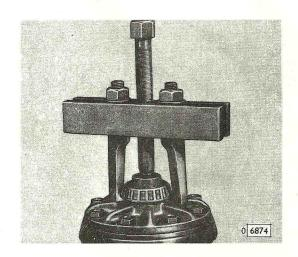
Unscrew ring gear bolts. With a brass drift strike off ring gear.
