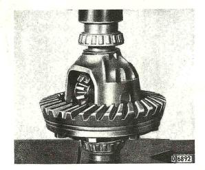
Install side bearings together with shims, using tool SW-221 (S-1206<sup>+</sup>).
