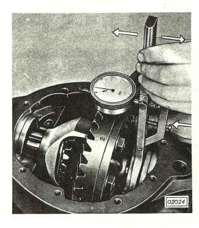
Check width at the four markings on ring gear to determine smallest width between differential case and rear axle housing. For control measuring rotate ring gear one turn in opposite direction to the previous rotation to the point with the smallest value.
