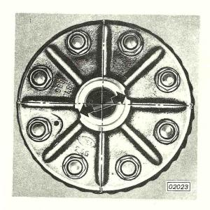
Mark four equally spaced points, numbered from 1 to 4 on ring gear circumference as shown in the illustration and carefully place differential case without roller bearings into split ring halves.
