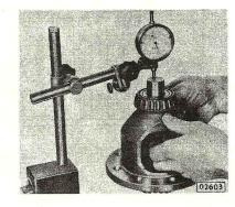
To obtain largest distance, revolve side gear several times.
