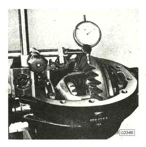
Check bearing preload. The bearings are properly preloaded, if the differential case can be pushed by hand three quarters of the way down in the bearing seats. The last quarter has to be equally seated by means of the bearing caps to a torque of 33 ft. lbs. (4.5 kpm).
