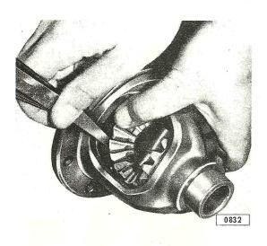
With a suitable drift drive pinion shaft out of differential case and take differential pinions and side gears out of differential case. If shims are installed, remove them too and, if necessary, replace them with new shims.
