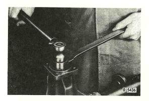
Counterholding with tool KM 106 (S-1288 +) unscrew drive pinion nut. With tool SW-209 carefully push drive pinion together with roller cage of inner bearing and clamp ring out of rear axle housing
