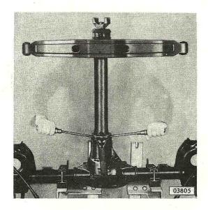
In case of excessive runout establish cause for runout, for instance dirt or burrs between contacting surfaces or bolts unevenly tightened.
