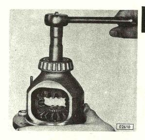
Check torque (fig. 02604) - permissible torque = 14 - 17 ft. lbs. (2-2.4 kpm).
