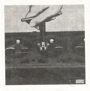
Vertically apply uniform pressure to cutters so that a concentric valve seat without chatter marks is obtained.
