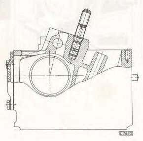
If after a short period of operation the valve clearance has abnormally changed, check stud tightness and retighten to specified torque.
