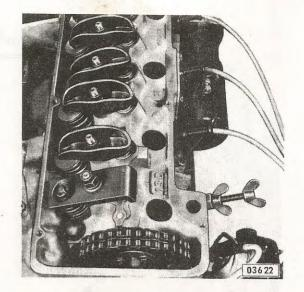
To avoid damage to the oil seal ring, first compress spring together with oil deflector and valve seat and then place oil seal ring in valve stem groove. This applies only to 16, 16 S and 19 S-engine. As far as the walve stem oil seals for 19 US-engines are concerned refer to page 06-45.
