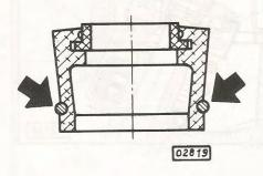
The Parts and Accessories Department supplies three versions of the oil seal according to the different valve stem diameters – standard and oversizes.
