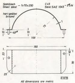
Deflect splash oil of timing chain with a protective metal sheet to be made up in own repairshop according to the dimensions given in the drawing. This metal sheet can also be obtained from Messrs. Matra-Werke under No. 0/58.
