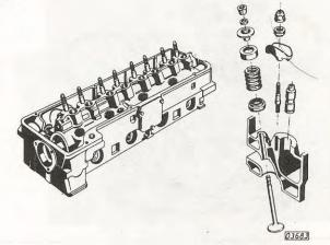
In order to obtain a proper and gas-tight valve seat, the intake and exhaust valves may be lapped with a fine-grained lapping compound.
