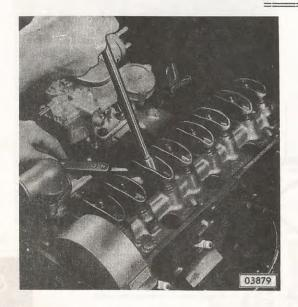
With engine at operating temperature (160° F = 80° C coolant and 140° - 160° F = 60° - 80° C oil temperature) adjust intake and exhaust valve clearance while engine is running to .012 in. (0.30 mm) by turning rocker arm nut. Feeler gauge should slide with a drag.
