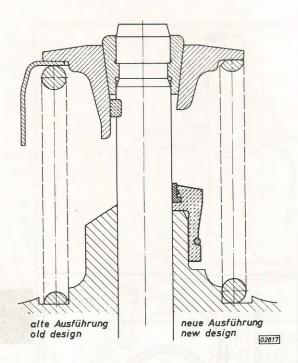
The right side of the illustration shows the valve stem oil seal of the 1.9 ltr. US-engine in installed condition (applies to intake valves only).
