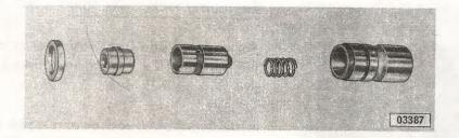
Oil escaping between plunger and lifter body and returning to the oil sump - this leakdown is necessary and desired - is always replenished due to the constant pressure when engine is running. A compensating spring in the pressure chamber above the plunger supports clearance-free valve operation.
