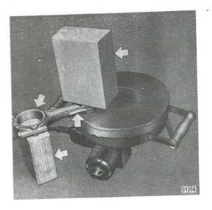
With the crayon a coloring substance is applied to the piston pin eye as well as the upper part of the connecting rod shaft. With its upper eye the connecting rod is then placed onto the heating plate. In order to obtain a quick and even heat flow, it has to be made sure that the eye surface planely rests on heating plate. For this purpose support opposite connecting rod end with a suitable block. To shorten the warm up period, it is advisable to place a fireproof clay onto connecting rod eye.
