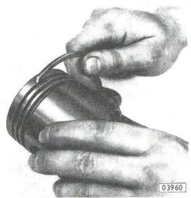
Decarbonize piston grooves using a piece of discarded piston ring.
