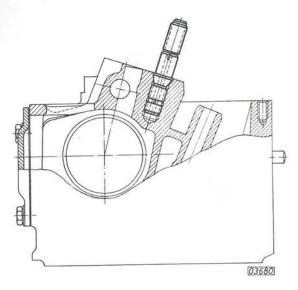
If after a short period of operation the valve clearance has abnormally changed, check stud tightness and retighten to specified torque.
