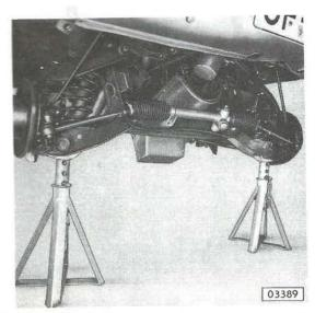
In this position support front suspension crossmember with stands and remove oil pan.
