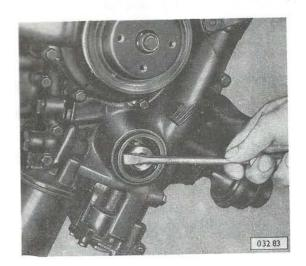
Remove crankshaft pulley.
