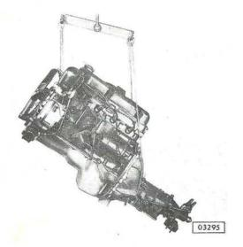
Lift engine so that engine supports clear the damper blocks. Bring engine in an inclined position and remove it from engine compartment.
