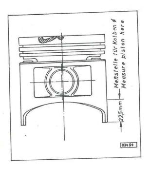
Select new piston according to table "Cylinder And Piston Dimensions".
