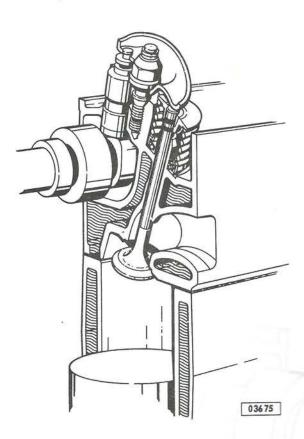
The head surface of the intake valves is no longer alutized. For this reason, the intake and exhaust valves may be lapped with a fine-grained lapping compound.
