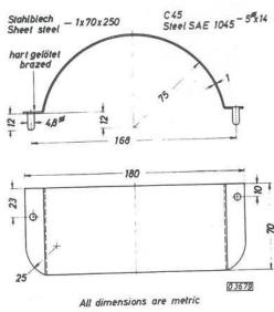
Deflect splash oil of timing chain with a protective metal sheet to be made up in own repairshop according to the dimensions given in the drawing. This metal sheet can also be obtained from Messrs. Matra-Werke under No. 0/58.
