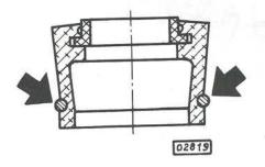
The Parts and Accessories Department supplies three versions of the oil seal according to the different valve stem diameters – standard and oversizes.
