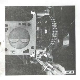
Prior to installation of cylinder head rotate crankshaft so that all pistons are positioned below U.D.C. When rotating crankshaft back and forth later on for attachment of cramshaft sprocket, it is absolutely necessary to loosen the adjusting nuts of the open valves so that valves do not touch piston heads.
