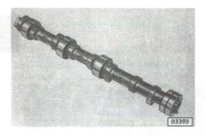
The cylinder head of the 1.9 ltr. US engines is equipped with a camshaft supported in four places.
