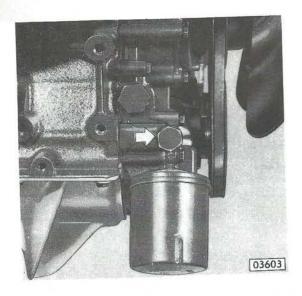
Unscrew plug and check spring and valve ball for free operation and dirt particles. If required, clean and free valve ball.
