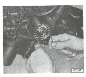
helical gear the distributor rotor must be in the same position as before, i.e. the notch on the rotor tip must be in alignment with the notch on distributor housing. Should this initial position not be obtained, remove helical gear from its seat again and stagger distributor driven gear one tooth by turning rotor accordingly. Check as to whether proper position has been obtained.
