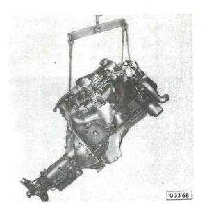
Place cables of engine lifter S-1220 around engine as shown in the illustration – short cable (59 in. = 1.50 m) in front and long cable (78.7 in. = 2 m) in the rear. Hook cables into hooks of engine lifter S-1220 and attach lifter to hoist. Ensure that no engine parts are damaged by cables.
