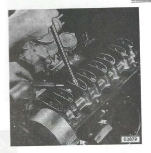
With engine at operating temperature (160° F = 80° C coolant and 140° - 160° F = 60° - 80° C oil temperature) adjust intake and exhaust valve clearance while engine is running to .012 in. (0.30 mm) by turning rocker arm nut. Feeler gauge should slide with a drag.
