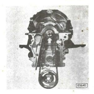
Make sure cramshaft sprocket mark is in alignment with mark on support and chain is in parallel with slipper pad. After sprocket has been fixed to camshaft, recheck alignment.
