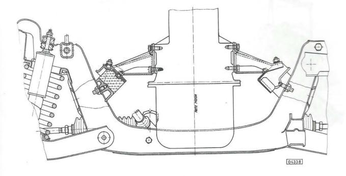
Unscrew nuts from threaded bolts of the engine support to damper block attachments.
