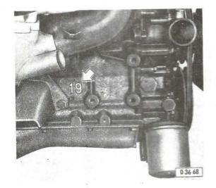
On installation of a new cylinder head attention has to be paid to the marking near the cover (see illustration)
