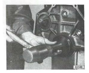
Drive in waved oil seal using tool S-1296.
