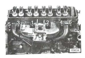
Retighten attaching bolts in cold condition after engine had reached operating condition.
