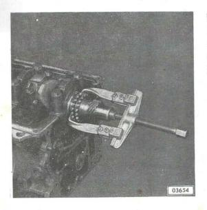
Remove chain and crankshaft sprocket. If required, use Kukko puller No. 20-1 together with thrust piece. If timing chain is to be reused, mark installation position.
