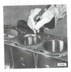
Pistons with index number "0.4" and higher are provided with oversize piston rings. On replacement of piston rings select them according to Parts Catalog specifications.
