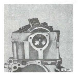
A nylon bolt in camshaft forward end serves to adjust end clearance.
