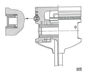
A PC-ring is used as oil control ring in lower piston ring groove.
