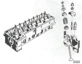
In order to obtain a proper and gas-tight valve seat, the intake and exhaust valves may be lapped with a fine-grained lapping compound.
