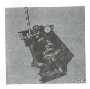
Check crankshaft for runout. Permissible runout should not exceed .001 in. (0.03 mm). To do this, remove center bearing shells so that crankshaft rests in front and rear main bearing shells. Check runout with dial gauge.
