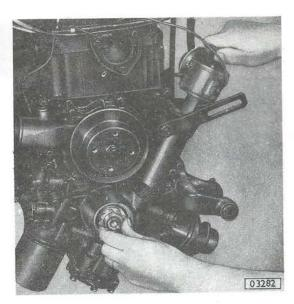
By turning rotor of distributor counterclockwise push helical gear on crankshaft journal outward, so that it can be pulled out by hand (helical gear has a sliding fit).
