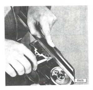
Check end clearance of gears. To do this, individually place gears without oil into pump and measure end clearance using a straightedge and a feeler gauge. Permissible clearance exists, if gear faces protrude 0 to .004 in. (0.10 mm) over cover contacting surface. Pump cover worn by gears must be replaced.
