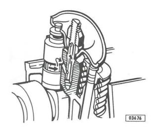
A squirt hole in connecting rod big end bearing splashes oil against right-hand side of cylinder wall. Additional cylinder wall and piston pin lubrication is through oil splash from crankshaft.
