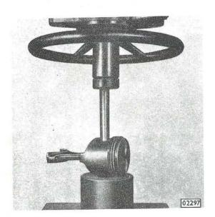
In cold condition press out piston pin, using tool S-1297 and a suitable support. Piston cannot be reused.
