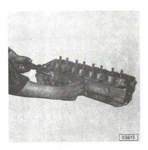
The Parts and Accessories Department supplies camshaft bearings for journals with .02 in. (0.5 mm) undersize only thereby providing replacement possibilities for all permissible dimensions (refer to respective table). If the required equipment is on hand, the desired bearing size can be made up in own repairshop.
