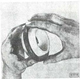
Place tapered ring with oil seal on crankshaft journal, snugly push oil seal over journal and remove tapered ring.
