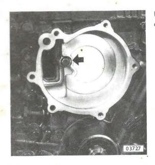
Unscrew timing case. Do not forget bolt covered by water pump.
