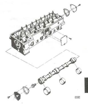
On installation of a new camshaft pay attention to marking on camshaft rear face.
