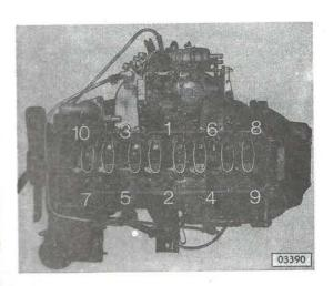
Place new cylinder head gasket without sealer, compensating gasket downwards, onto cylinder block. Install cylinder head assembly and tighten bolts on cold engine in the sequence shown in the illustration to a torque of 72 ft. lbs. (10 kpm), using tool MW 110.
