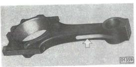
As soon as the connecting rod eye has reached a temperature of 536° F (280° C) the applied coloring substance is getting black indicating the desired assembling temperature. The color line should not change color over its entire length but only up to the beginning of the connecting rod shaft.
