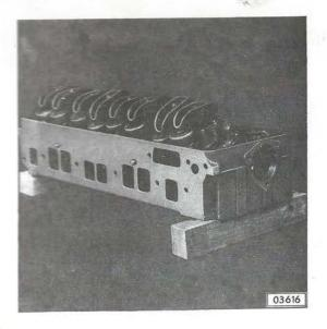
Always use two suitable wooden blocks to support cylinder head, if it is placed on work bench assembled with camshaft and valves. Otherwise valves held open by camshaft would touch work bench and valve shafts may get distorted.
