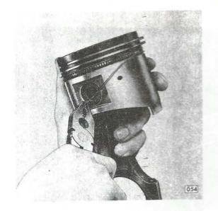
On installation first place intermediate ing into groove, making sure that ring gaps are not superjacent. Then, one after the other, spirally install upper and lower seel band ring, reversing removal opera-
