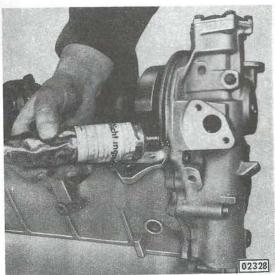
Prior to reinstallation of oil pan coat contacting surfaces of oil pan cork gaskets and rubber strips on cylinder block side with sealing compound, part No. 15 03 161, and install cork gaskets. Fill gaps at the gasket ends with sealing compound, part No. 15 04 402, and place rubber strips into grooves. Install oil pan.
