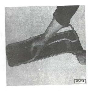
Button cork gasket onto rocker arm cover - do not cement it to cover.
