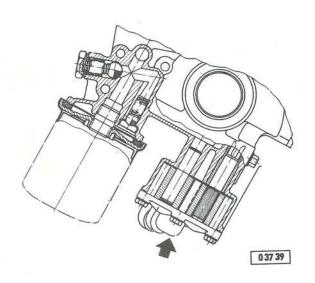
The oil pump pressure regulator valve of the 1.9 ltr. US-engines is located in the oil pump cover. If the oil pump cover was removed, make sure on reinstallation that the plug points to vehicle rear end.
