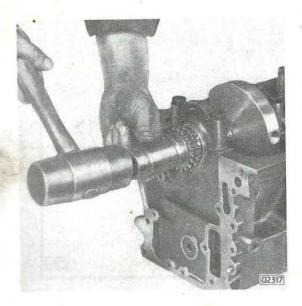
With a suitable sleeve drive sprocket, onto camshaft journal paying attention that key is properly seated.
