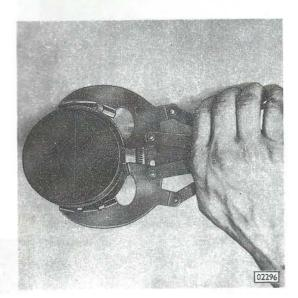
Remove and install piston rings, using piston ring pliers (except oil control ring).
