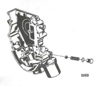
In case of symptoms caused by insufficient oil pressure - oil pressure indicator lamp lights up - always check oil pump pressure regulator valve for proper operation.
