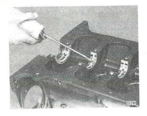
Prior to installation of crankshaft fill oil gallery of cylinder block with engine oil.
