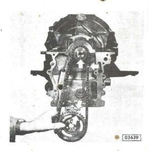
With tool S-1305 press new seal ring into timing case paying attention that timing case is not damaged. Lightly coat seal ring seat with sealer, part No. 15 04 167.
